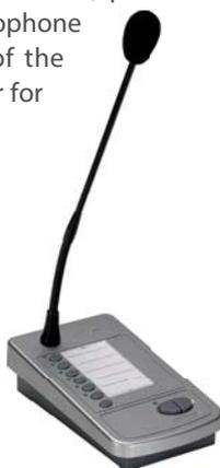
**PMB112-G | Pre-amplified unit** with 12 programmable zone push-buttons and associated indicator LEDs, an All-Call key, a hold-down call key (PTT), a toggle button (LOCK) for long messages and a microphone activated and busy LED.
