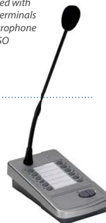
**PMB106-G | Pre-amplified unit** with 6 programmable zone push-buttons and associated indicator LEDs, an All-Call key, a hold-down call key (PTT), a toggle button (LOCK) for long messages and a microphone activated and busy LED.
